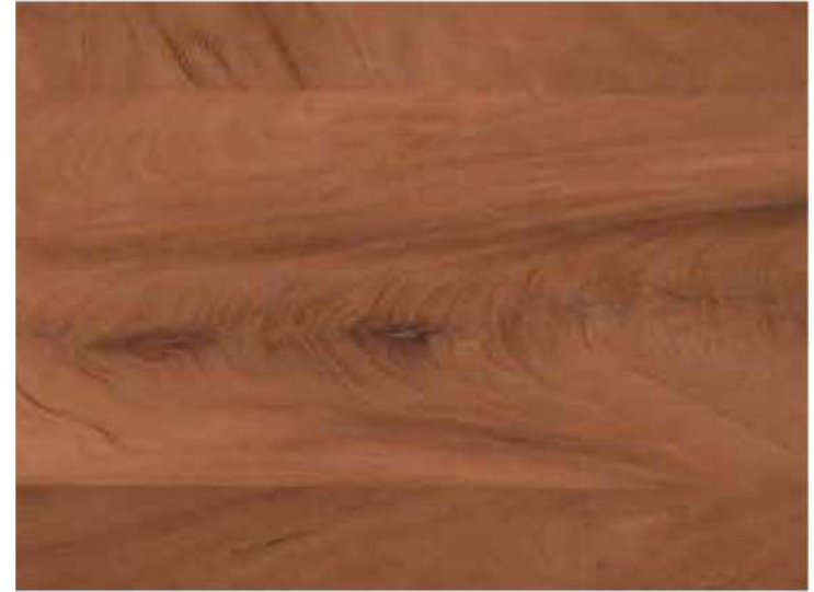
The intersection of a branch with the main section which causes a grain pattern is known as a crotch. The cross section of this leads as a beautiful section in the grain.
